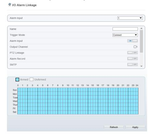
Step 2 Choose alarm input and trigger mode, set name, enable other linkages such as alarm input, PTZ linkage, Alarm Record, SMTP, FTP upload and so on.
