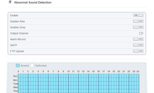
Step 2 Enable the audio abnormal detection, enable sudden rise, sudden drop, when happen the condition of enable, it will alarm.
