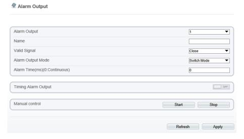
Step 2 Set alarm output of channel, name, enable valid signal and alarm time choose alarm output mode.
