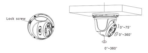
Step 5 After the adjustment of location, then tighten the lock screw, tighten the decorative cover following as the arrow direction and finish the installation.
