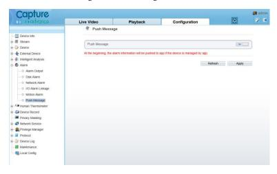
Step 2 Enable the push message, you will receive the message when the alarm happened. Step 3 Click **Apply** to save the settings, click **Refresh** will return last settings.
