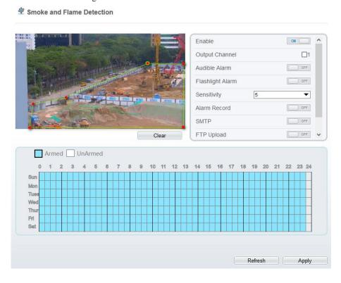
Step 2 Set all parameters for smoke and flame detection. Table 7-2 describes the specific parameters.
