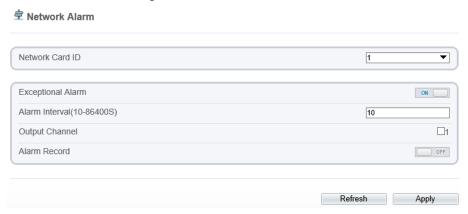
Step 2 Choose network card ID and enable exceptional alarm to set alarm interval. Tick output channel.
