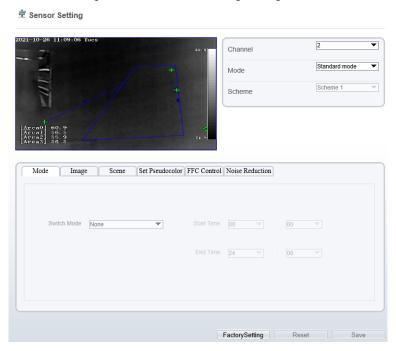
Step 2 Choose **Channel 2**. The thermal channel **Image Settings** is displayed. Step 3 Choose the scheme from drop-down list, there are four schemes can be setting.
