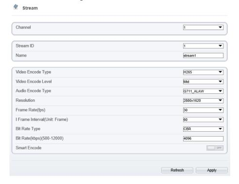
Step 2 Choose channel, stream ID, video encode type, video encode level, audio encode type, resolution, frame rate, frame interval, bit rate type and bit rate from all drop list.
