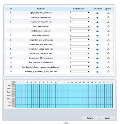
User can set the audio file manually. Click to upload the audio file(The type should be WAV, size must be less than 250 Kb, the bit rate should be 128 kbps.), as shown in Figure 3-13.
