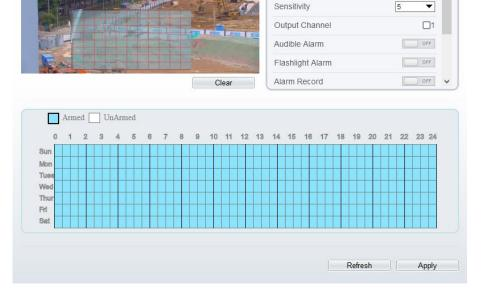
Step 2 Choose channel and enable the motion alarm, set alarm interval and sensitivity, output channel, alarm record, audible alarm, flashlight alarm, enable other linkages such as SMTP, FTP upload and so on.
