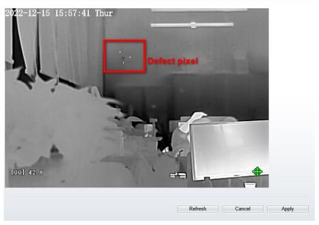
Step 2 Click the white point at image, click **Refresh** to recover the defect pixel, as shown in Figure 3-17.
